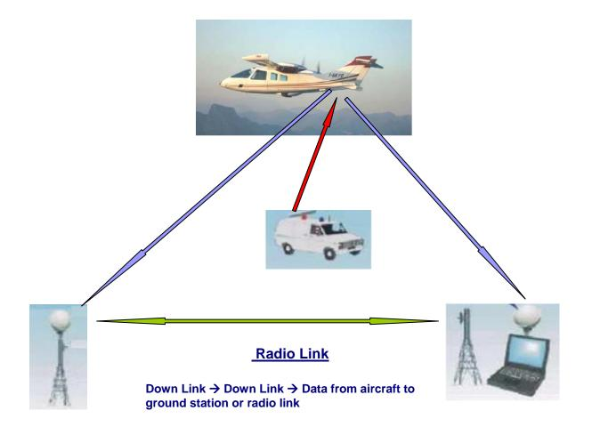
UP Link → From Mobile Station to Aircraft (Coverage Area → 30 Km max)
