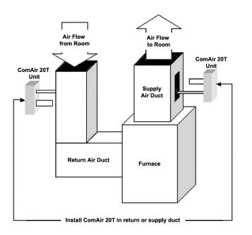
The ComAir 20T may be installed either in the main return duct or main supply duct as shown in the diagram. When installing on the supply side, locate it as far away from the heating source as practical while remaining in the main air stream.
